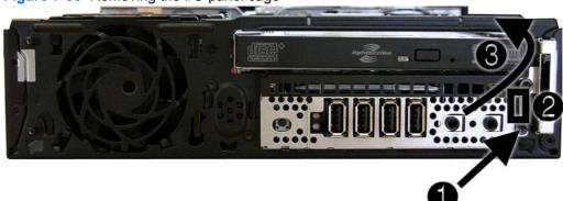
Figure 7-35 Removing the I/O panel cage
